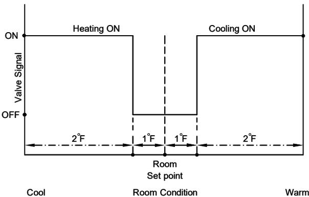
**Sequence of Operation -- On/Off Heating or Cooling with Heat/Cool Changeover**
