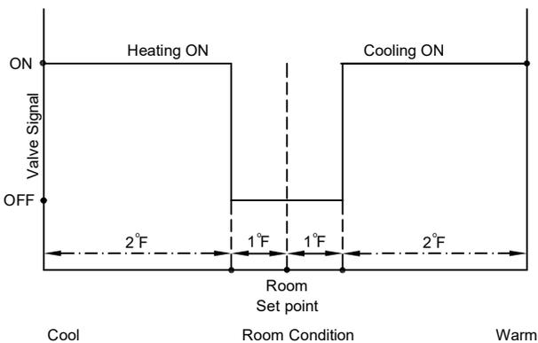
**Sequence of Operation -- On/Off Heating & On/Off Cooling**
