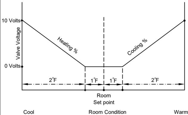
**Sequence of Operation -- Modulating Heating or Cooling**
